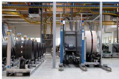
Ferag delivered a second RollSertDrum inserting drum, several MultiDisc unwinding stations for the automatic assignment of preprints and main products, and a second RollStream line with JetFeeder feeders.
